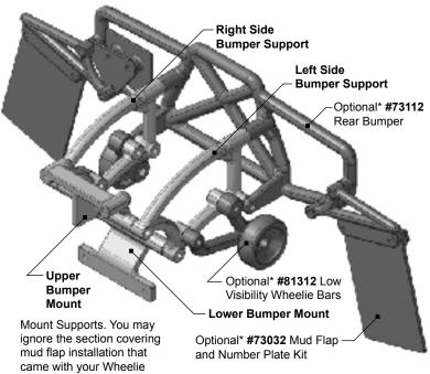
Bars. For reference, an optional\* *RPM* Mud Flap and Number Plate Kit is available for the SCTE (*RPM* #73032). However, they mount to the optional\* *RPM* SCTE Rear Bumper (*RPM* #73112) as shown in the illustration above.
